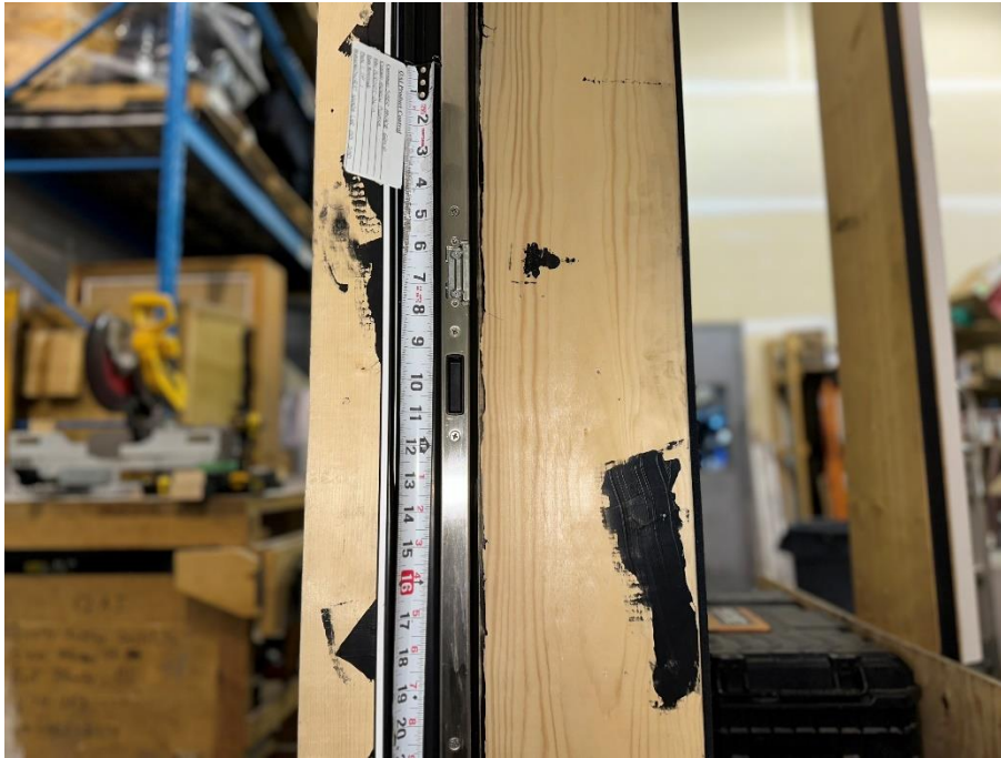
Figure 23: I-bar keeper system – Lower middle section.
