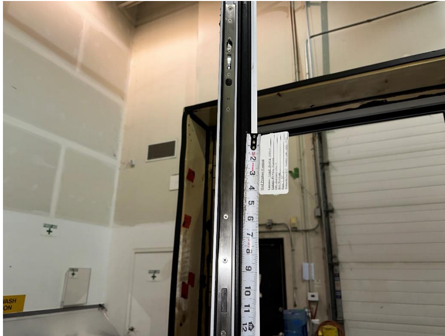
Figure 21: I-bar locking system – Upper Section.
