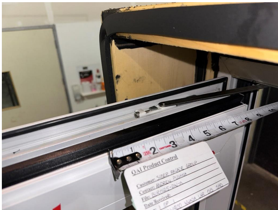
Figure 28: Stay arm hinge – Door slab side.
