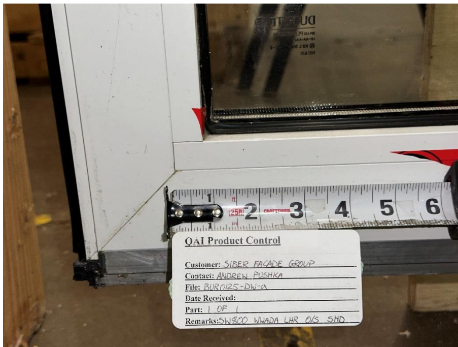
Figure 6: Glazing bead corner joint.
