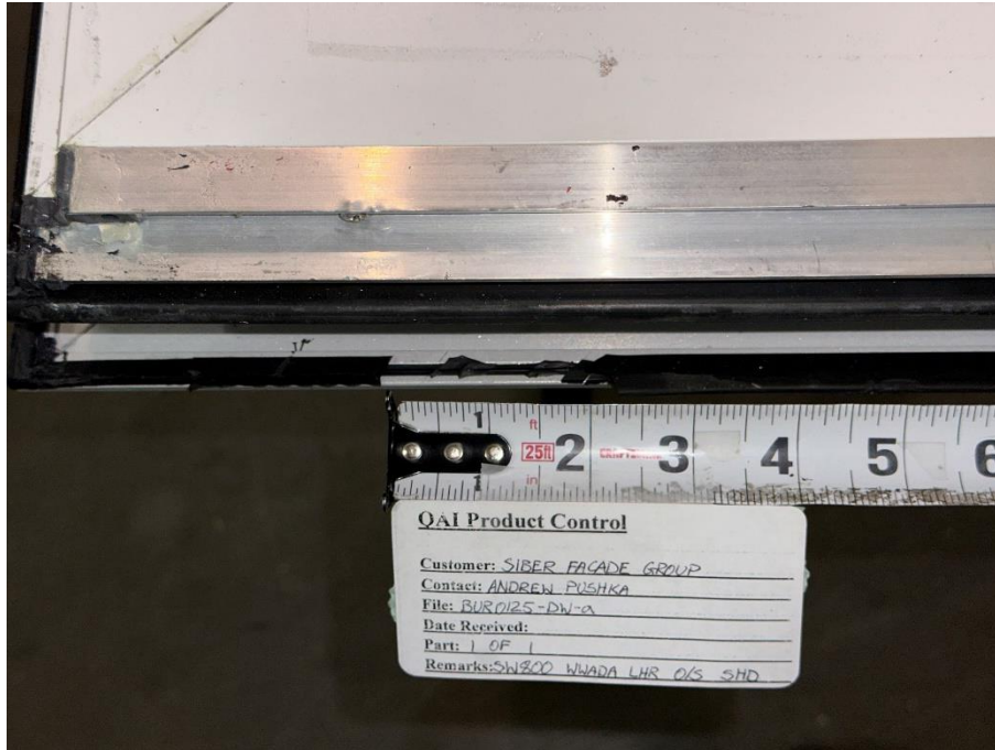
Figure 17: Notch in door slab weather-stripping for drainage.
