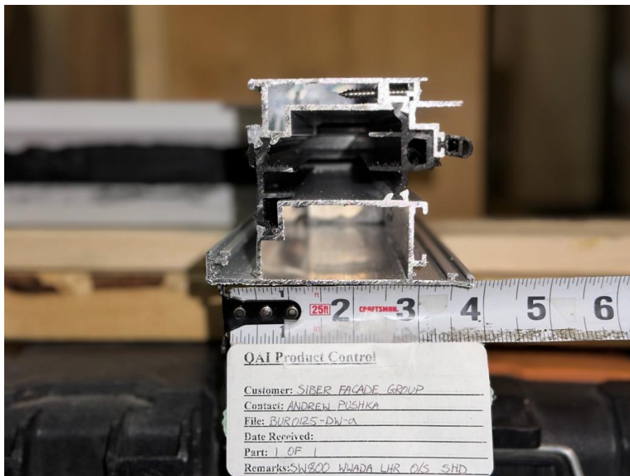
Figure 4: Door slab – Bottom rail.
