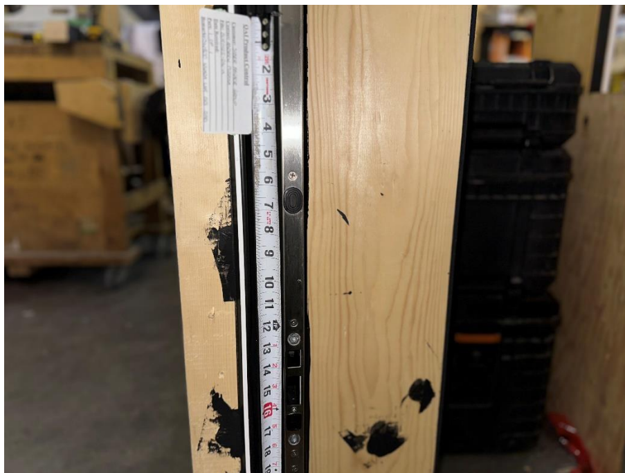
Figure 22: I-bar keeper system – Lower section.
