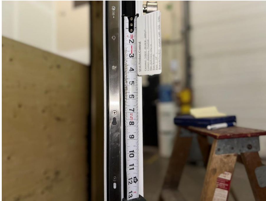
Figure 19: I-bar locking system – Lower Middle section.
