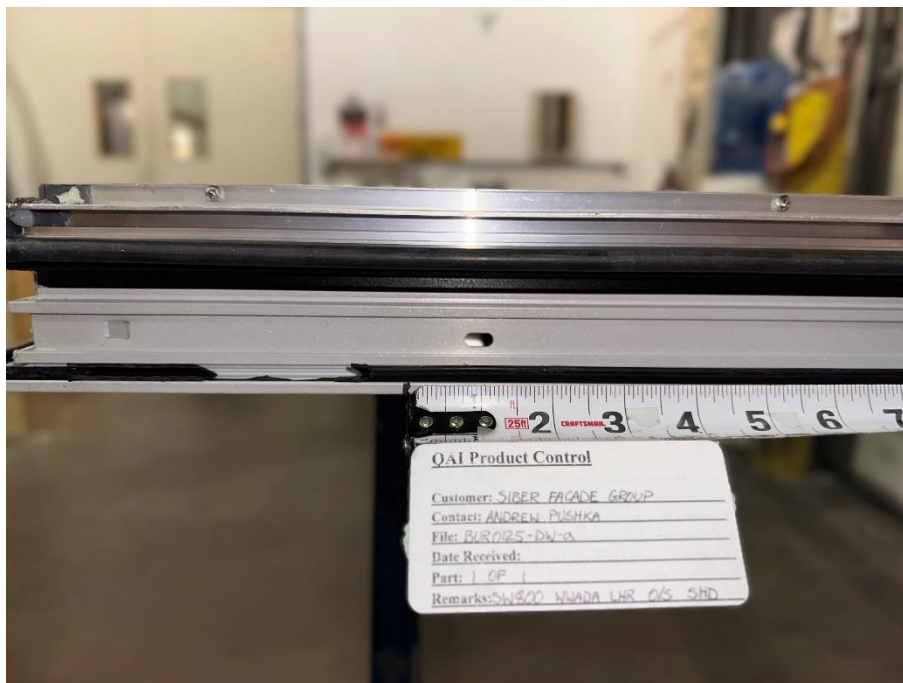
Figure 16: Drainage out of the door slab.
