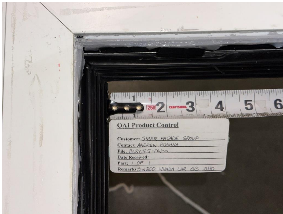
Figure 14: Exterior glazing gasket corner joint.
