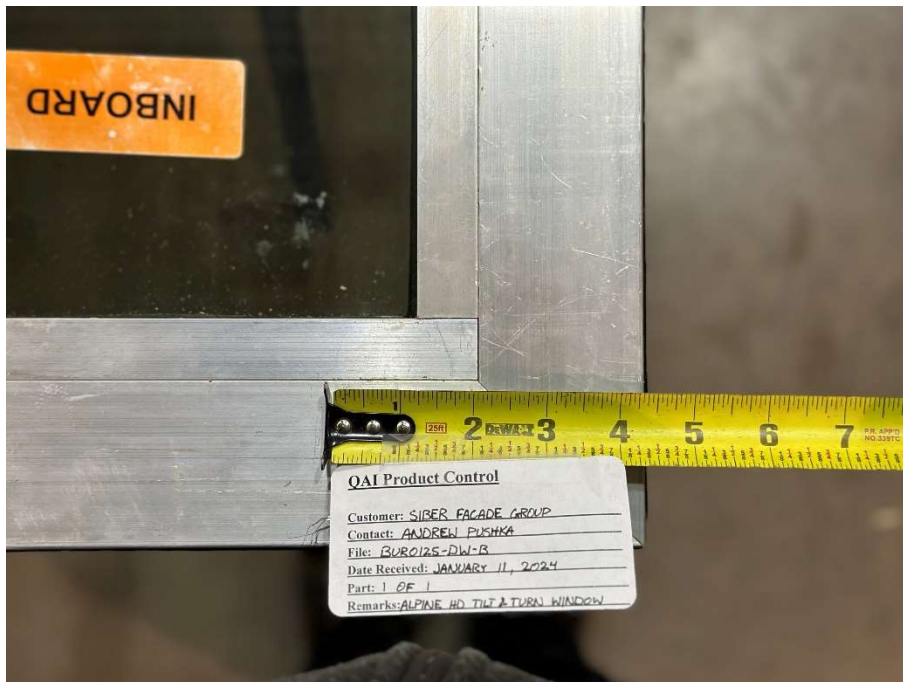
Figure 4: Glazing bead corner joint.
