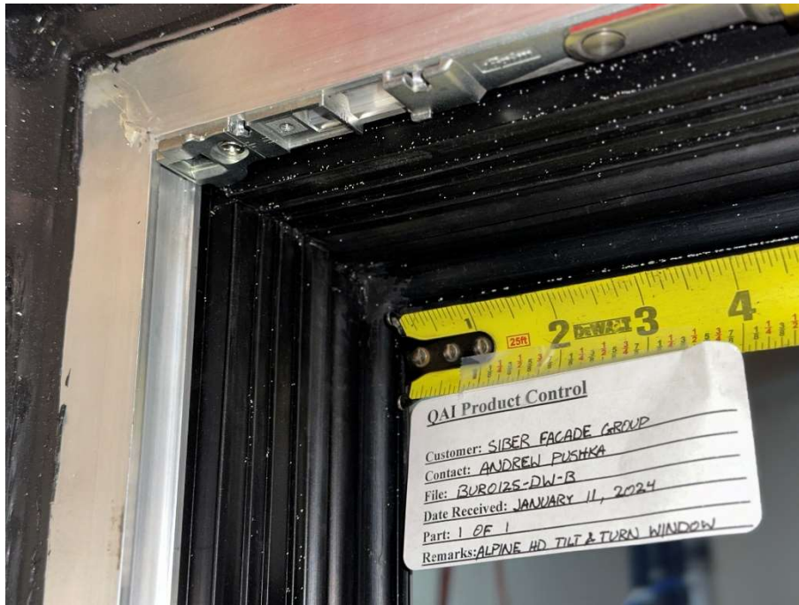
Figure 7: Weather-stripping joints - Frame.
