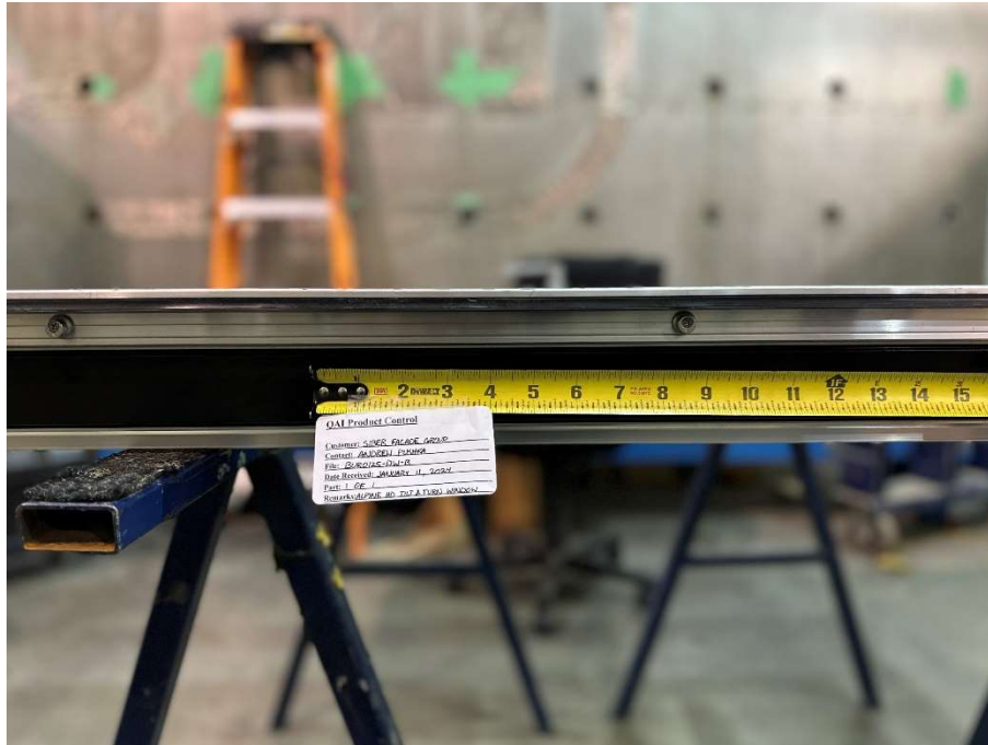
Figure 29: Multi-point locking system - Hinge stile - Middle section.
