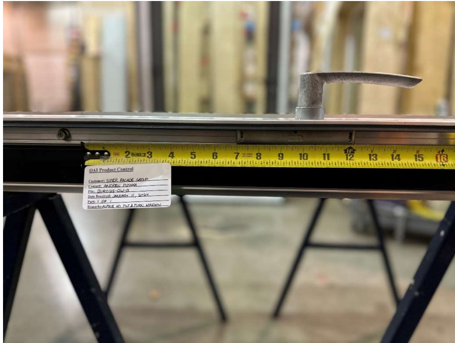
Figure 23: Multi-point locking system - Locking stile - Middle section.
