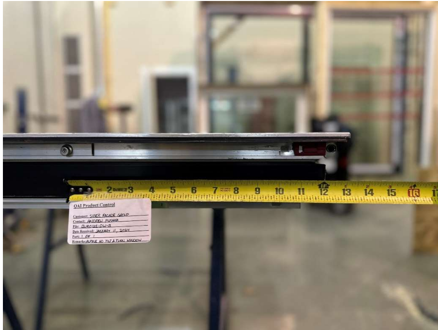
Figure 27: Multi-point locking system - Bottom rail - Hinge side section.
