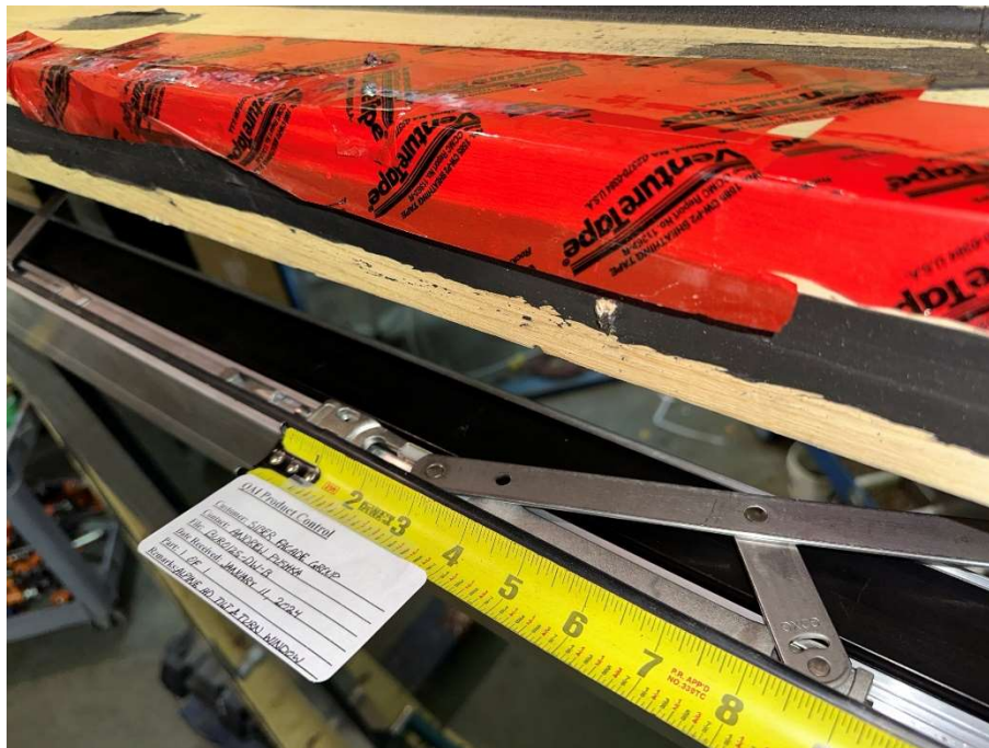
Figure 18: Casement/stay arm hinge - Sash side.
