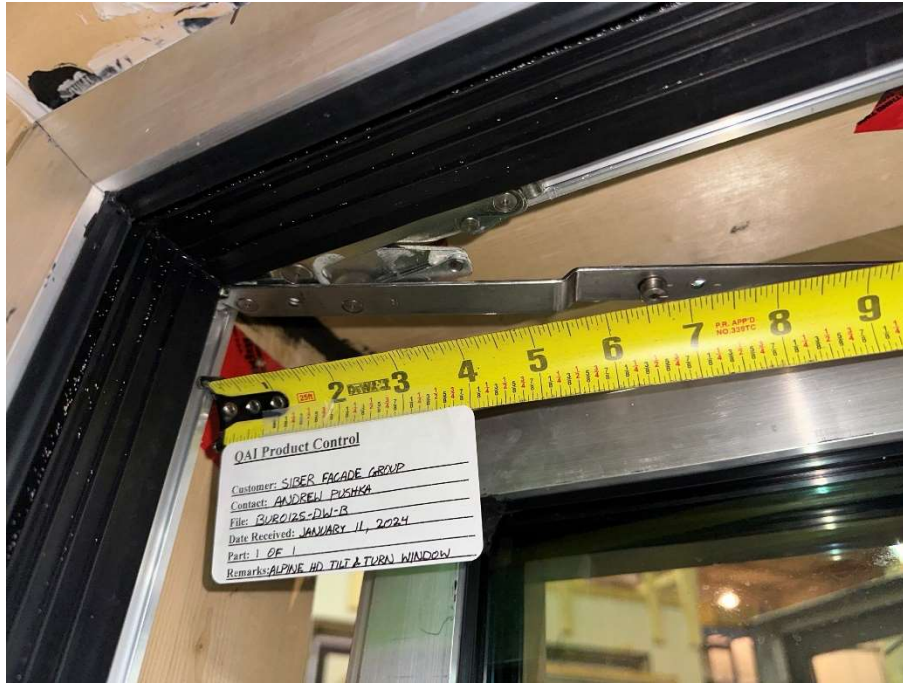
Figure 17: Casement/stay arm hinge - Frame side.
