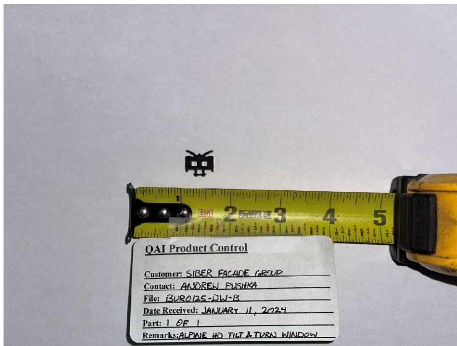
Figure 10: Exterior glazing gasket.
