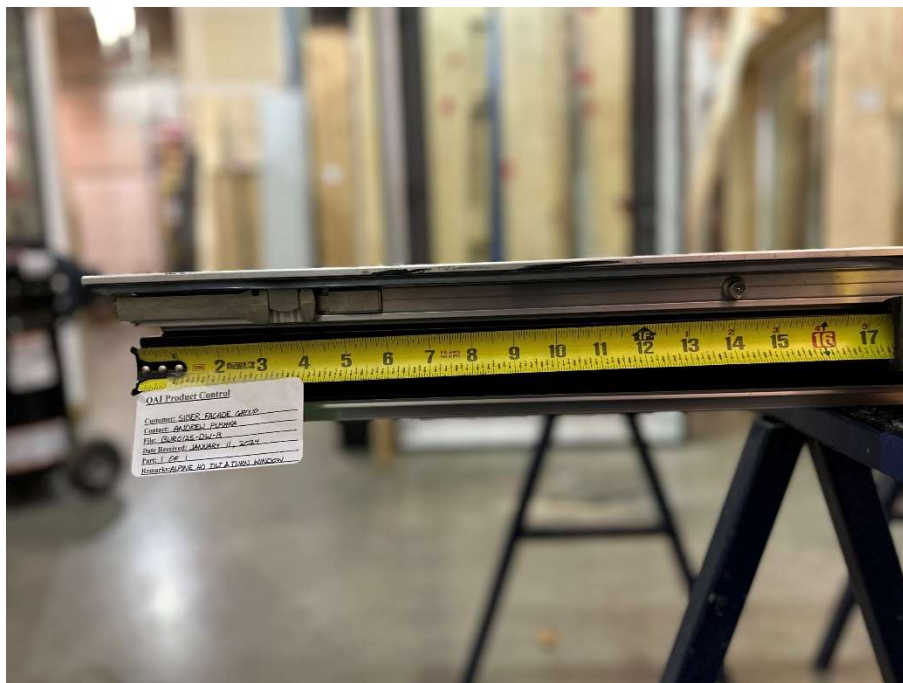
Figure 22: Multi-point locking system - Locking stile - Upper section.
