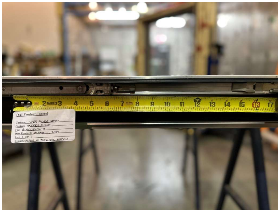
Figure 20: Multi-point locking system - Top rail – Middle section.
