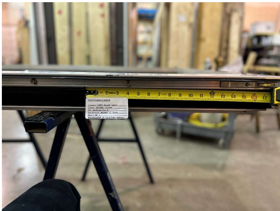
Figure 24: Multi-point locking system - Locking stile - Lower section.
