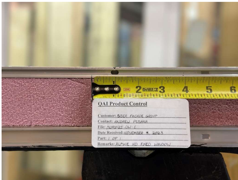
Figure 6: Drainage out of the frame.
